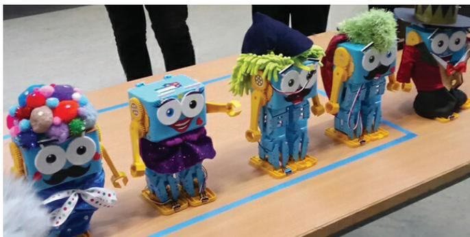
The Marty<sup>15</sup> robot can be programmed to move and dance, and it also has built-in sensors. This means it can be programmed to respond to different conditions. After learning how to instruct the robot to move around based on distances and angles, they could then tell it to move until a condition is met, such as moving forward until it bumps into a wall!
